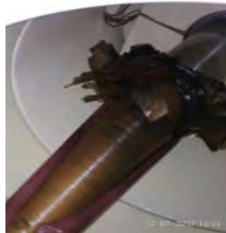
Fig 3,,4 and 5 show the commonest of failure causes : the bushing failures at some of the installations.
